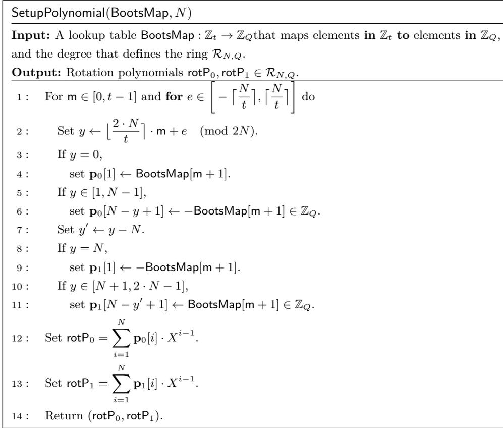
**Figure 3:** Algorithm to set up the rotation polynomial based on a look up table
