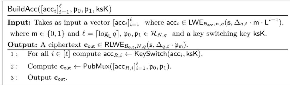
Figure 2: Accumulator builder algorithm.
