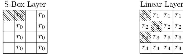
**Figure 4:** Examples of what an adversary can observe in the masked MIDORI (similarly in SKINNY and PRINCE) by placing a probe in a masked S-box pair or in the linear layer. We include the dynamic randomness (with  $r_4 = r_1 + r_2 + r_3$ ) which is added after the layers.
