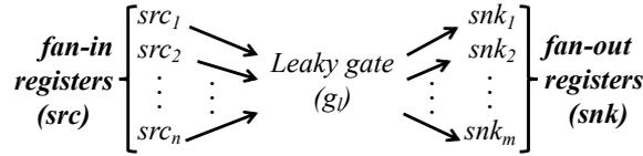
**Figure 6:** NGA uses fan-in and fan-out registers for each gate to determine its approximate location in the design.
