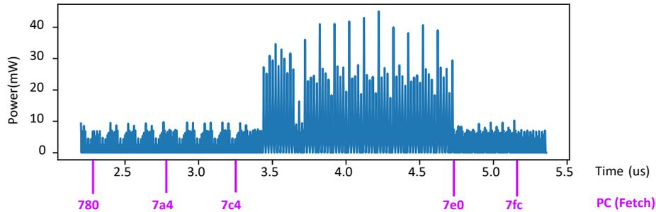
**Figure 8:** (Example 1) Average simulated power trace for SoC programming and running the AES hardware accelerator. The bottom X-scale links the power trace to Listing 1 through the value of the program counter (Fetch stage).
