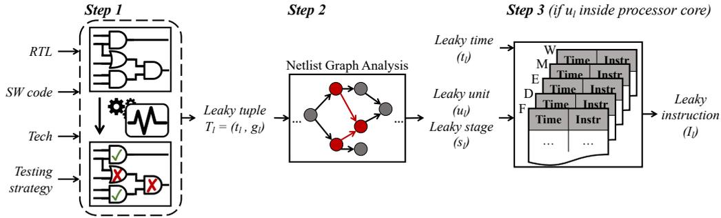
Figure 2: Overall RootCanal flow
