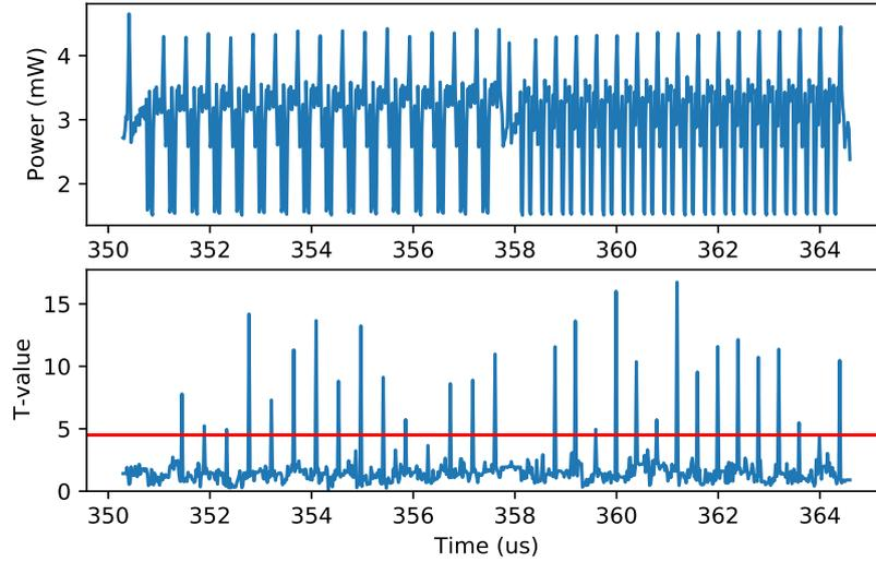
**Figure 10:** (Example 3) Average simulated power trace and TVLA result for the byte-masked AES example
