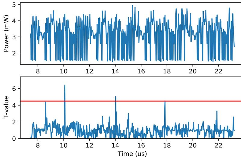
**Figure 12:** (Example 4) Average simulated power trace and TVLA result for bit-sliced masked PRESENT SBox
