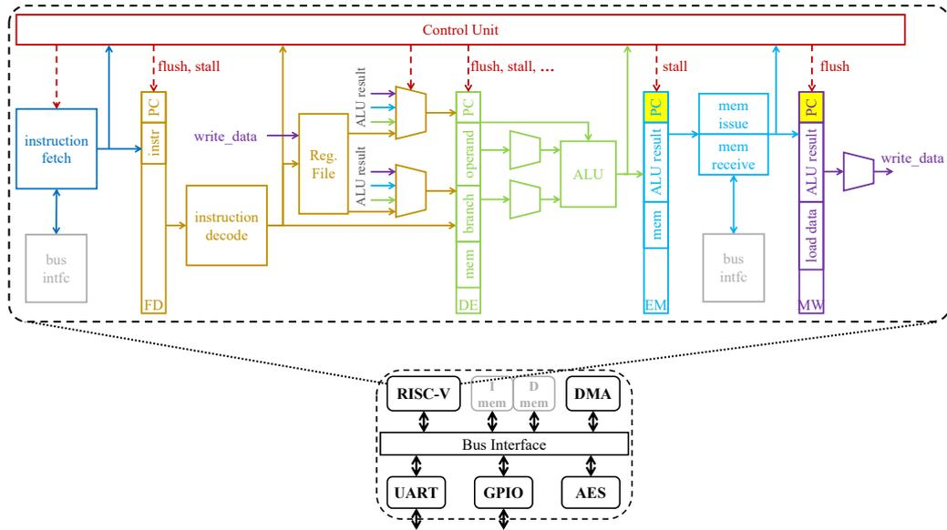
**Figure 3:** Block diagram of RISC-V-SoC and its five-stage RISC-V processor. Resources from different pipeline stages are shown in different colors in the processor core. The gray blocks in the SoC (instruction and data memories) are modeled in the testbench (not synthesized).
