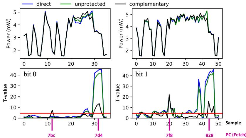
**Figure 9:** (Example 2) Average simulated power traces and TVLA results for redundant encoding schemes on bit-sliced PRESENT SBox
