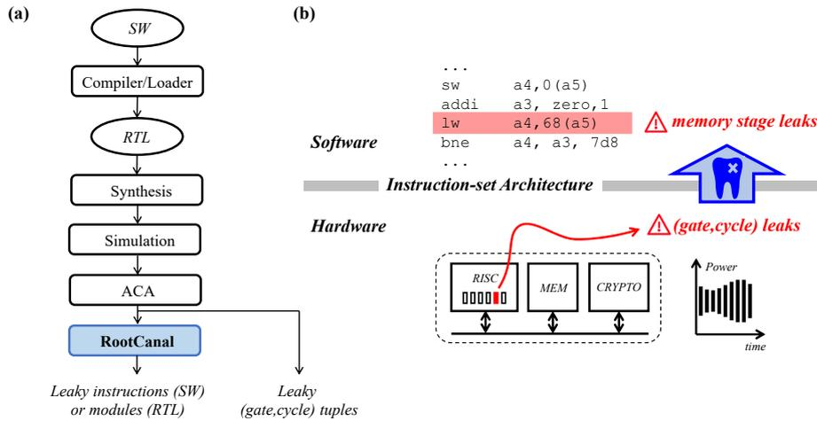
**Figure 1:** RootCanal is a pre-silicon side-channel leakage assessment technique to back-annotate leaky (gate,cycle) tuples in an SoC design to high-level software or hardware information. (a) RootCanal design flow integration (b) Example application.
