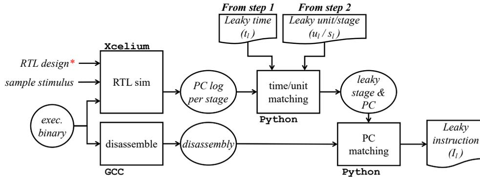
**Figure 7:** Layout of step 3 in RootCanal. The RTL design may need to be modified to pass on the PC signal to all pipeline registers. The executable binary is generated in the same way as in step 1.
