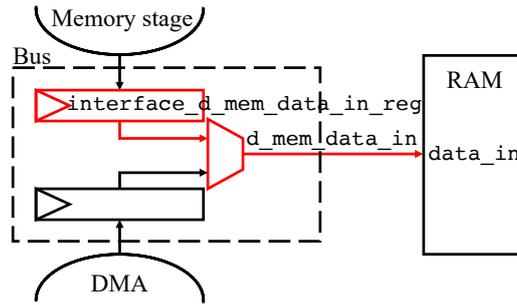
**Figure 11:** Leaking circuit in byte-masked software AES
