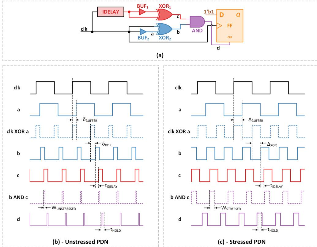
**Figure 3:** Working Principle of PPWM Sensor Showing (a), Labeled Block Diagram; (b), Waveforms for Unstressed PDN; and (c), Waveforms for Stressed PDN.
