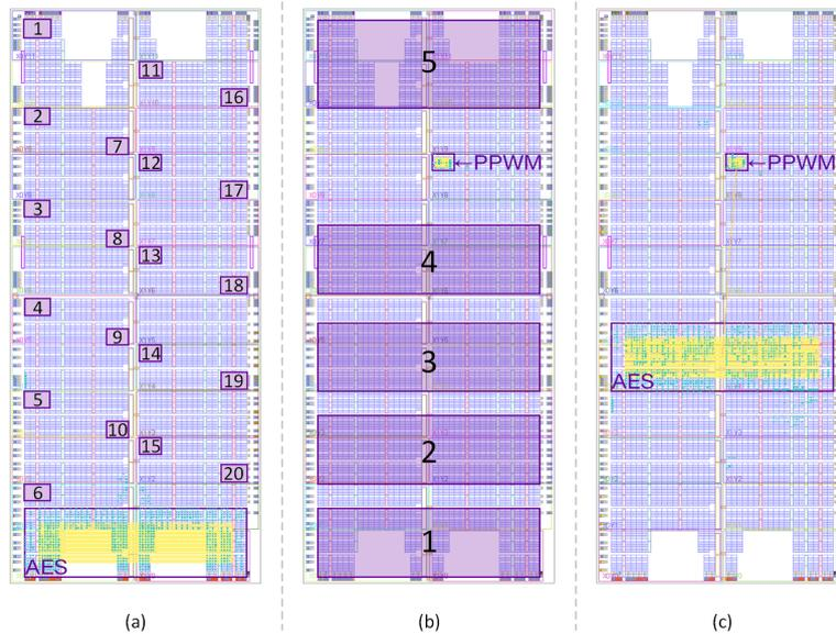
**Figure 7:** (a) - (c) PPWM and AES Module Placements on the Floorplan of SAKURA-G Main FPGA Used in Experiment Setup I.
