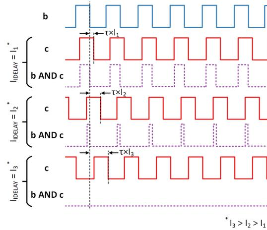
**Figure 4:** Calibrating  $t_{IDELAY}$  with CONTROL\_FSM.
