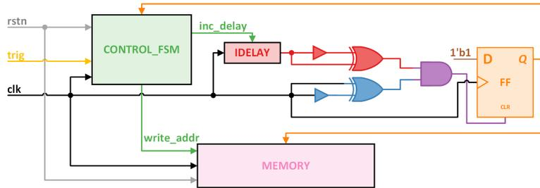
**Figure 2:** The Abstract Design of the Proposed PPWM Sensor.
