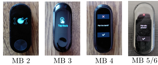
Figure 3: Mi Bands pairing confirmation messages. To accept pairing, a user must either press a hardware button (Mi Band 2/3) or touch a software button (Mi Band 4/5/6). Note that Amazfit Cor 1/2 use similar pairing confirmation messages.
