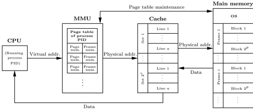
**Figure 1:** Components involved in the memory management of conventional modern computer systems [And19].
