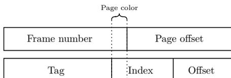
**Figure 4:** Physical-to-cache address translation in physically indexed caches [VKM19].
