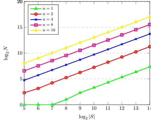
**Figure 5:** Rekeying periods  $N$  so that  $\mathcal{C}$  is  $N$ -access secure with advantage at most 0.01, where  $|S|$  denotes the number of cache sets and  $a$  the associativity.
