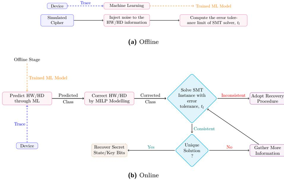
**Figure 1:** Schematic of work-flow of our side channel attack framework
