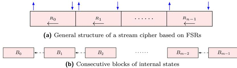
**Figure 3:** Internal state and its block representation
