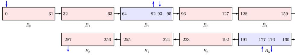
**Figure 7:** State registers of TRIVIUM (split into blocks of 32 bits)
