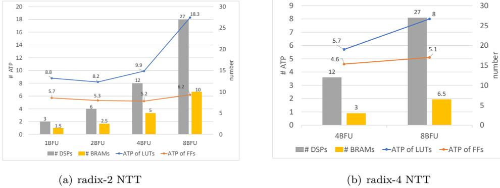
**Figure 12:** The variation of ATP in radix-2 and radix-4 NTT ( $N = 1024$ , 14-bit  $q$ ).
