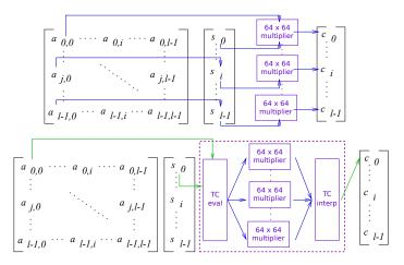
**Figure 1:** Comparison of parallel polynomial multiplication in Espada (top) with polynomial multiplication in Saber (bottom). The lines in blue and green denotes parallel and serial execution respectively. The components inside the boxes are implemented on hardware.
