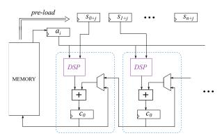
**Figure 4:** Architecture of the compact  $64 \times 64$  polynomial multiplier used for Espada
