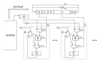
Figure 5: Parallel architecture of Sable polynomial multiplier
