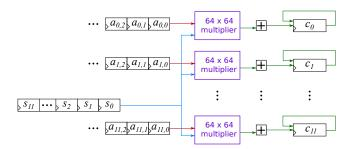
Figure 3: Parallel architecture for matrix-vector multiplication in Espada
