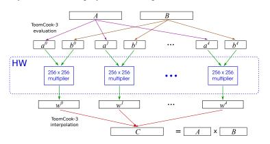
Figure 2: Proposed HW/SW partition for a Florete accelerator
