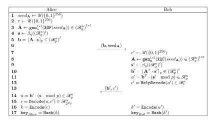
Protocol 1: A generalized key-exchange scheme based on LWR
