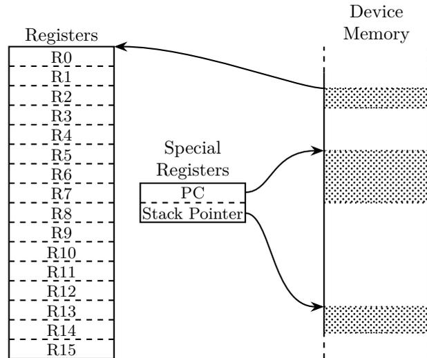
**Figure 11:** Visualization of a Generic VM Structure.
