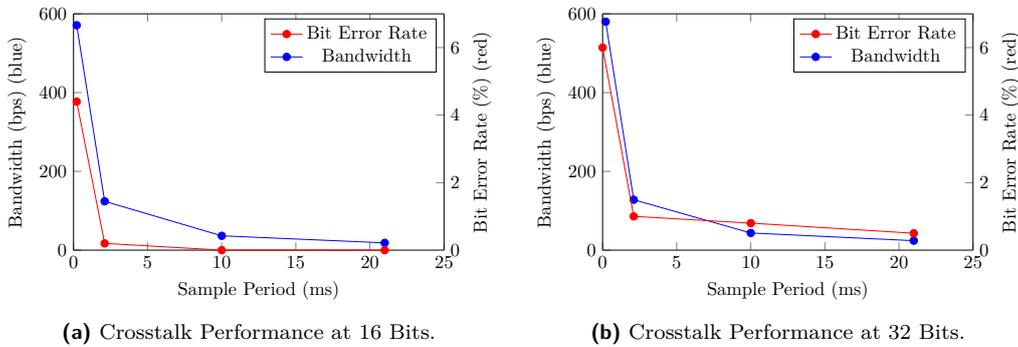
**Figure 9:** Crosstalk Evaluation. Transmission Bandwidth (blue) and BER (red) for Data Transmitted in 16- and 32-Bit Chunks. 8-Bit CRC Included with Each Chunk.
