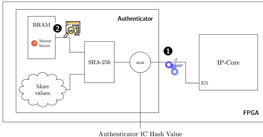
**Figure 2:** Overview on the FPGA Authentication using an Authenticator IC.
