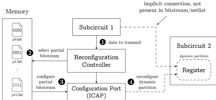
**Figure 5:** Setup for Covert Communication with Partial Reconfiguration.
