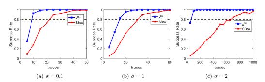
**Figure 14:** The success rate of deep learning based profiling attacks on simulated leakages with different noise levels.
