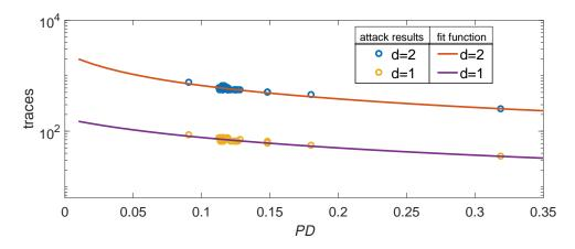
**Figure 4:** Number of traces for the GE to be below 10 (in y-axis) versus the different *PD* (in x-axis) for n = 8 and  $\sigma = 0.1$ .
