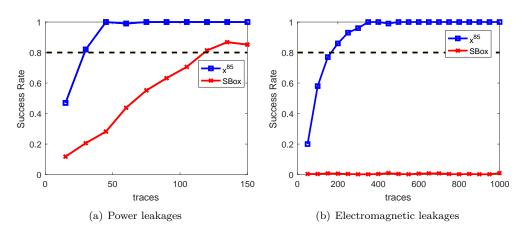
Figure 15: The success rate of deep learning based profiling attacks on practical leakages.
