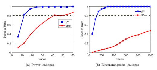
Figure 13: The success rate for ETA on practical leakages.
