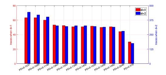
**Figure 3:** Number of traces for GE to be below 4 (in y-axis) versus the different *PD* (in x-axis) for n = 6 and  $\sigma = 0.1$ .
