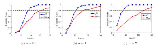
**Figure 12:** The success rate for ETA on simulated protected leakages with different noise levels.
