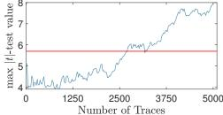
**Figure 1:** A first-order RvR test on the unprotected Picnic3 implementation using revealed values from the offline phase. The traces are classified based on the bit  $\lambda_1^w + \cdots + \lambda_{16}^w$ . Values above the 5.7 threshold (red line) indicate strong leakage (left). Moreover, the maximum |t|-value increases with respect to the number of traces and the leakage becomes clear after 2,725 traces (right).
