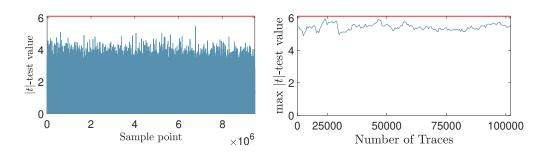
**Figure 4:** A first-order leakage detection test based on 100,000 traces on the Picnic3. The |t|-value remains below 6.1 (as suggested by [DZD<sup>+</sup>18]), indicating the absence of exploitable first-order leakage for the 100,000 traces. Also, the maximum |t|-value is bounded and becomes stable with the increased number of traces (right).
