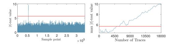
**Figure 5:** A first-order RvR test on the unprotected Picnic3 implementation using revealed values from the online phase. The traces are classified based on a single bit of  $\hat{sk}K_0$ . Values above the 5.7 threshold (red line) indicate there are strong leakages (left). Also, the maximum |t|-value increases with respect to number of traces and the leakage becomes absolute after 6,000 traces (right).
