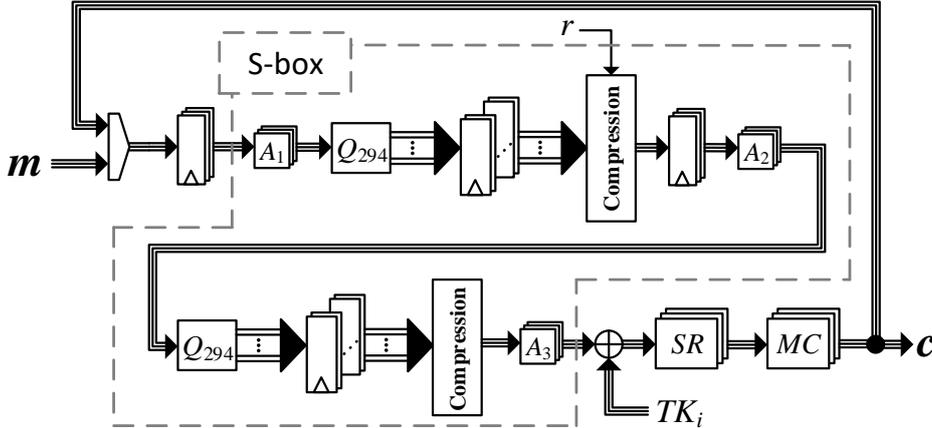
**Figure 2:** Design architecture of our round-based second-order SKINNY-64 encryption function.
