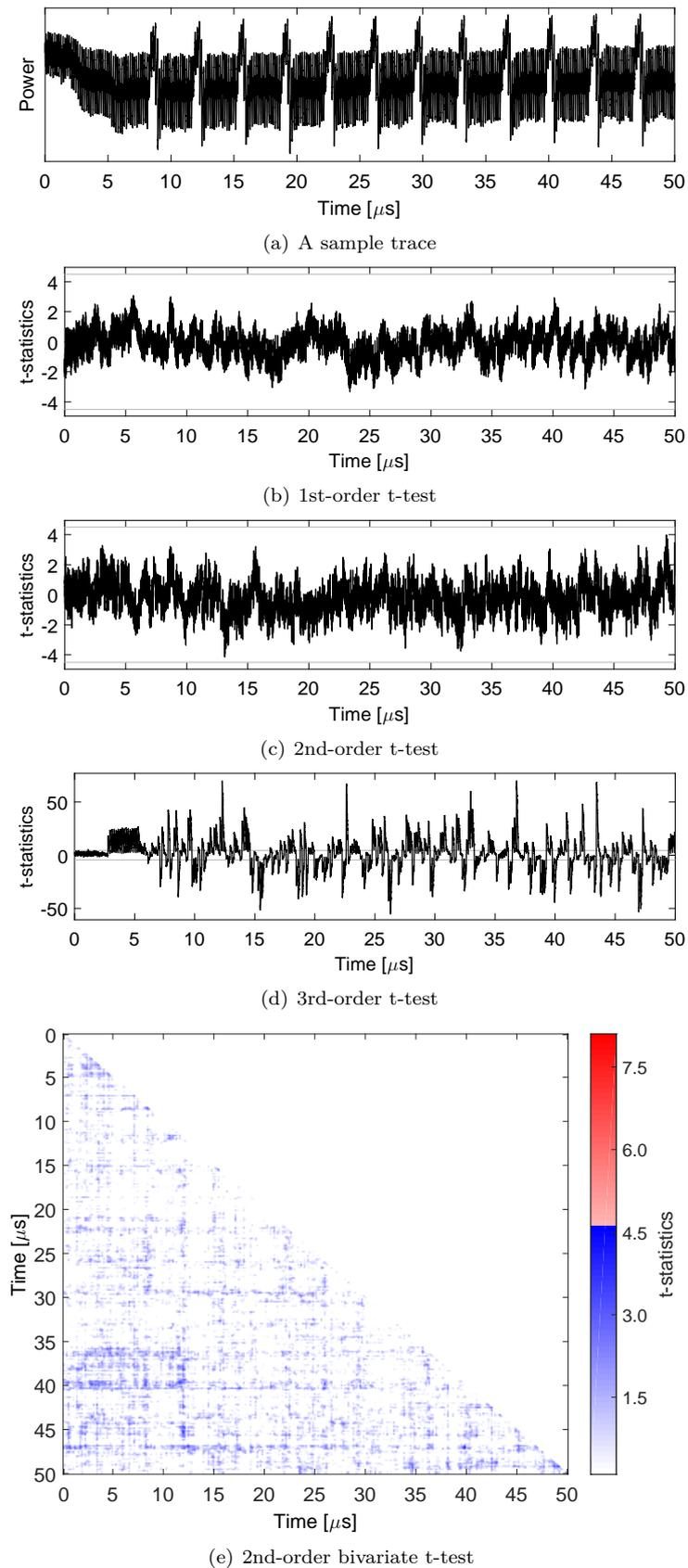
**Figure 10:** Experimental analysis of our second-order secure round-based PRESENT encryption design, 100 million traces.
