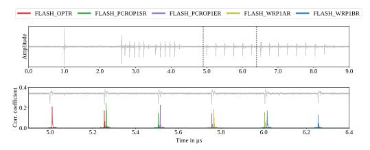
**Figure 6:** EM trace during the boot phase of an STM32L4 microcontroller (top). The zoom (bottom) of the region between the two dashed lines shows the results of a correlation-based leakage test on the option byte registers with 200 000 traces.
