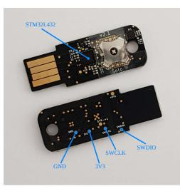
**Figure 4:** Front (top) and back side (bottom) of the SoloKeys Solo. The integrated microcontroller and the accessible supply and debug pins are highlighted.
