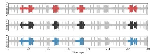
**Figure 5:** EM traces of the first ladder step of the attacked token (middle) and the oracle with k set to 0 (top) and 1 (bottom). Regions where distinctive patterns from the oracle trace match with the token are highlighted in blue and red otherwise.
