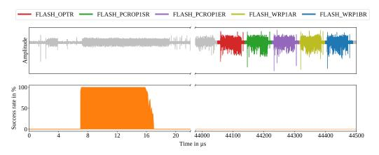
**Figure 7:** EM trace (top) and success rate of an injected glitch (bottom) during an RDP downgrade to level 0. The write operations of the option bytes are highlighted in color.
