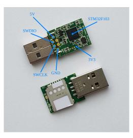
**Figure 3:** Front (top) and back side (bottom) of the Nitrokey Pro 2. The integrated microcontroller and the accessible supply and debug pins are highlighted.
