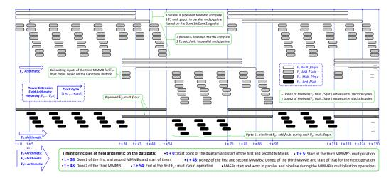
**Figure 9:** Timing diagram and scheduling technique of the tower extension field arithmetic operations (i.e.,  $\mathbb{F}_p$ ,  $\mathbb{F}_{p^2}$ ,  $\mathbb{F}_{p^4}$ ,  $\mathbb{F}_{p^6}$ , and  $\mathbb{F}_{p^{12}}$  arithmetic) in our datapath [BJ20a].
