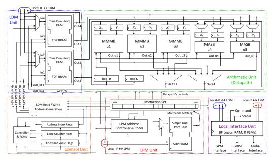
Figure 2: Architecture details of the CP core.
