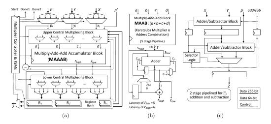
Figure 8: Structures of (a) MMMB, (b) MAAAB, and (c) MASB blocks [BJ20a].
