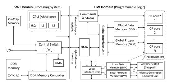
Figure 1: High level architecture of the programmable HW/SW codesign accelerator.
