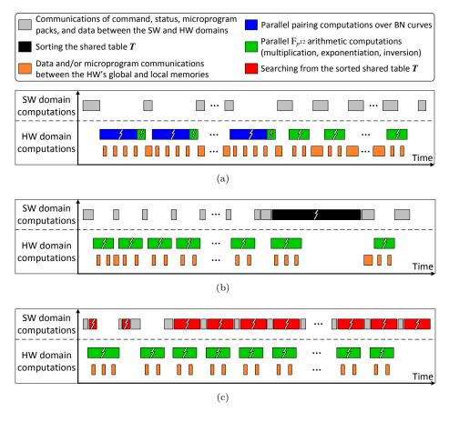
**Figure 4:** Implementation and timing diagrams of (a) the parallel pairings and  $\mathbb{F}_{p^{12}}$  arithmetic computations of Alg. 1 (i.e., lines 1-6), (b) the precomputation part of Alg. 4(a), and (c) the on-the-fly computation part of Alg. 4(b).
