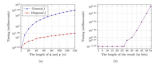
**Figure 5:** Timing results of the HW/SW codesign for (a) pairings and  $\mathbb{F}_{p^{12}}$  arithmetic (Alg. 1 lines 1–6) as a function of n, the length of  $\mathbf{x}$  and  $\mathbf{y}$ , and (b) discrete logarithm (Alg. 1 line 7) as a function of the length of the result in bits.
