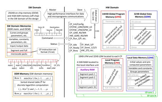
Figure 3: Memory taxonomy and interaction principles of the SW and HW domains.
