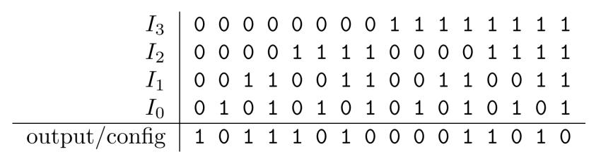
• These configurations can be read from the bitstream of an FPGA.
