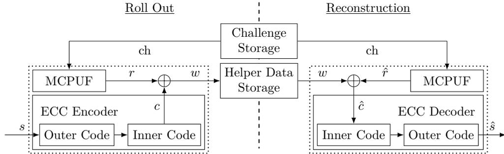
**Figure 1:** Visualization of the key-storage scenarios with PUFs: At some point in time – during *Roll Out* – a key is stipulated for the device. Later – during *Reconstruction* – the key is derived from the noisy PUF given public helper data and challenges.
