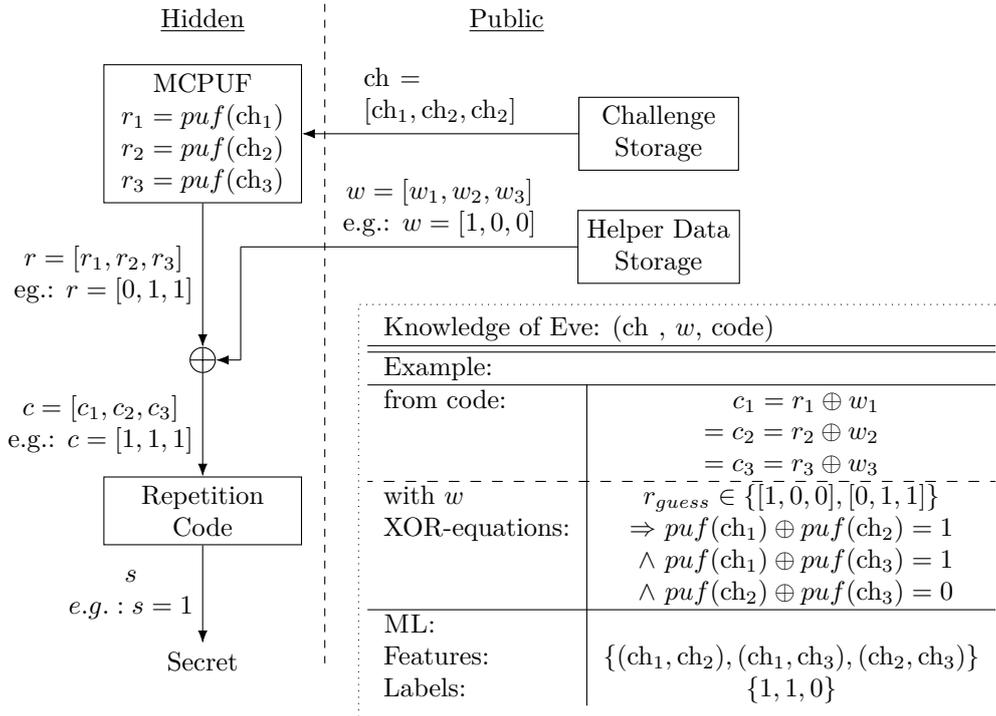
**Figure 2:** Visualization of the attacker knowledge using a (3,1,3)-repetition code. The left side is hidden from E; Public information and its exploitation is given on the right.
