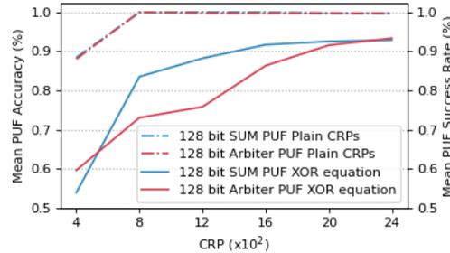
**Figure 10:** Comparison between mean PUF accuracy for learning a 128 bit APUF and a 128-SUM PUF through CRPs and PUF success rate when learning the same PUFs through HD.
