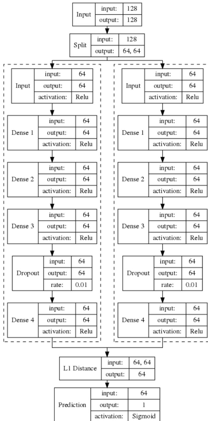
**Figure 12:** SNN used to learn PUFs using XOR equations derived by a repetition code. During training the loss is calculated using binary cross entropy. The chosen optimizer is Adam with default parameters and a learning rate of 0.01.
