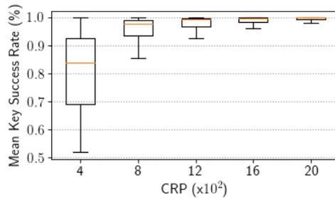
**Figure 5:** Mean key success rate of the ML model for a 128-SUM PUF based on measured frequency data.
