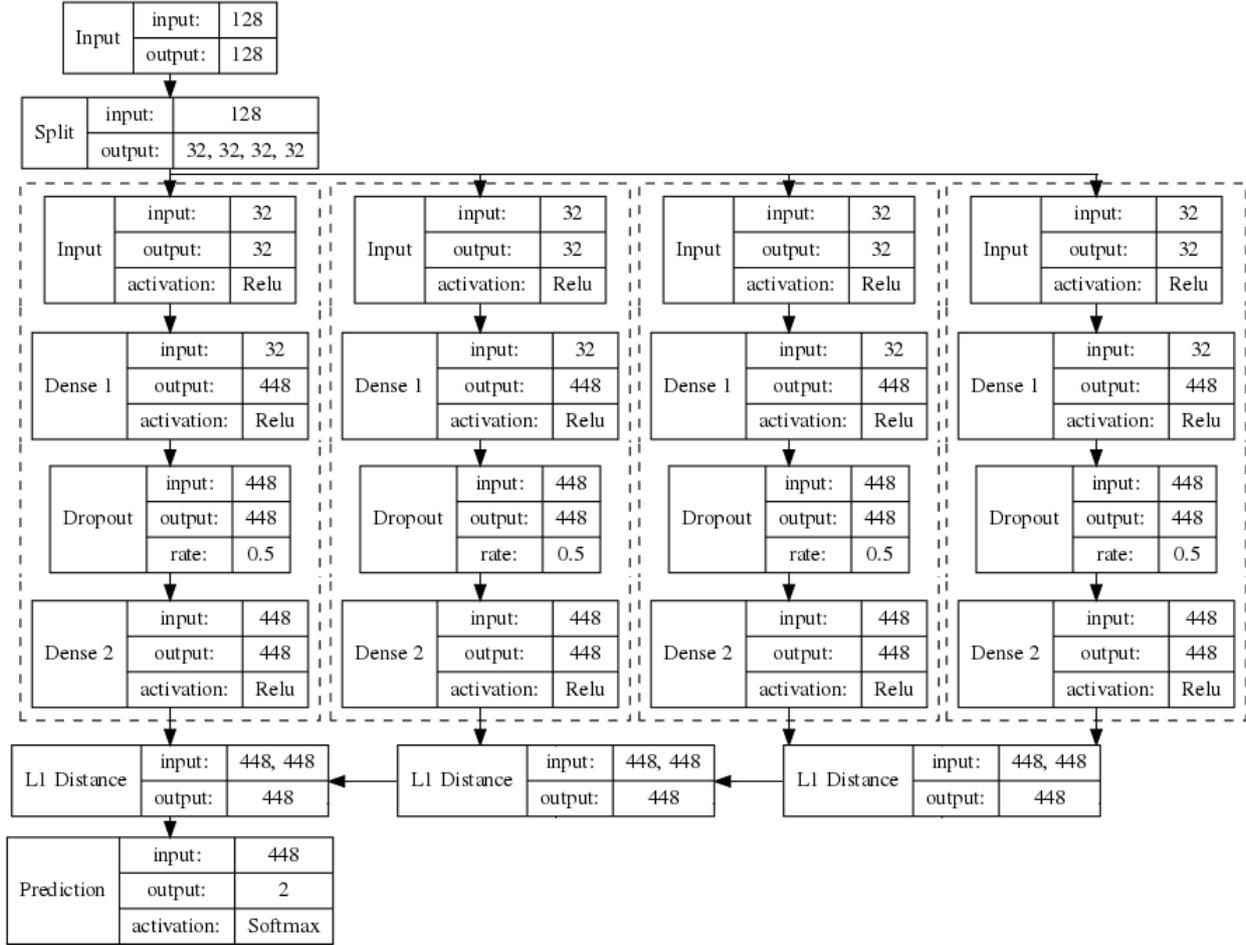
**Figure 11:** SNN used to learn PUFs using XOR-equations derived by SPC, BCH and RM codes. During training the loss is calculated using sparse categorical cross entropy. The chosen optimizer is Adam with default parameters and a learning rate of 0.001.
