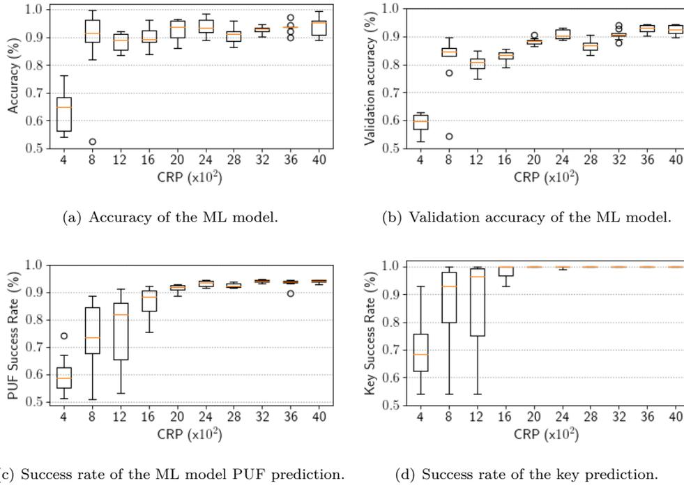
**Figure 4:** Evaluation of the attack idea using a repetition code with  $n = 7$ , Arbiter PUF model with 128 bit challenge, and a Siamese neural network. For every number of CRPs ten neural networks were trained and evaluated.
