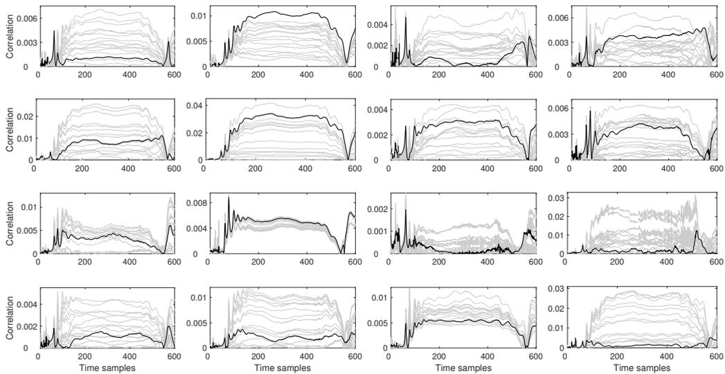
**Figure 14:** MCDPA attack on unrolled PRINCE using 100 million traces when the plaintext is reset to a random state between encryptions. Results for 16 key differences (0-1, 1-2, ..., 14-15, 15-0) are presented.
