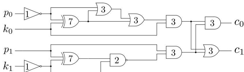
**Figure 1:** Toy encryption circuit with two plaintext inputs  $p_0, p_1$ , two key inputs  $k_0, k_1$  and two ciphertext outputs  $c_0, c_1$ . The numbers within the logic gates denote their propagation delay in time delay units ( $tdu$ ).
