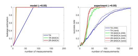
**Figure 8:** Leakage bounds and success rates of experimental SASCA with up to two rounds against an unprotected AES implementation in a known plaintext scenario (I).
