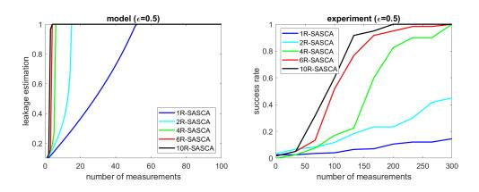
**Figure 10:** Leakage bounds and success rates of experimental SASCA with up to ten rounds against an unprotected AES implementation in a unknown plaintext scenario.
