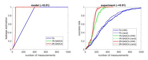
**Figure 9:** Leakage bounds and success rates of experimental SASCA with up to two rounds against an unprotected AES implementation in a known plaintext scenario (II).
