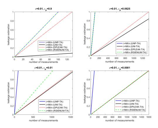
Figure 17: Leakage bounds for shuffled implementations.
