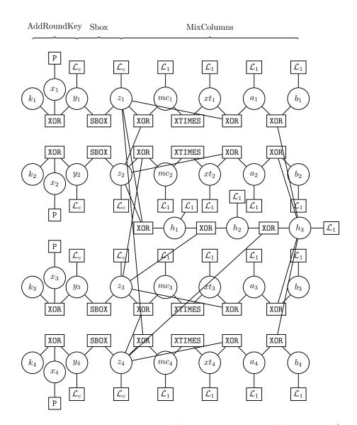
Figure 5: Factor graph for the first round / first column of the AES (adapted from [GS15]).
