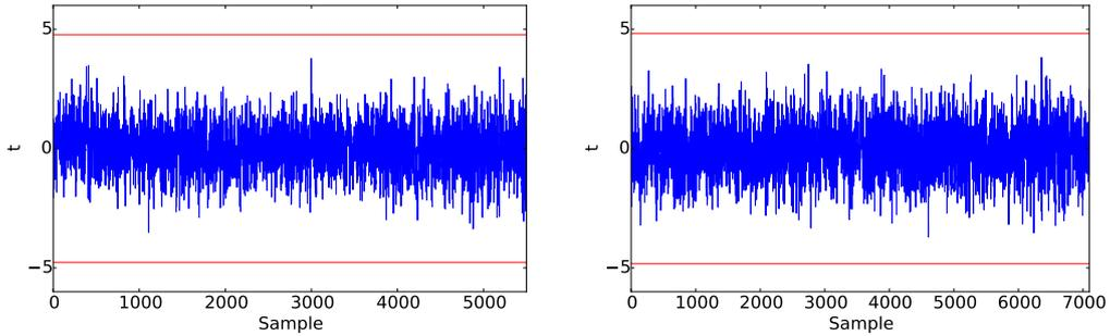
**(a)** First-order leakage for two-share version with four coefficients (masks enabled, 1 M measurements,  $t_{th} = 4.77$ ).
