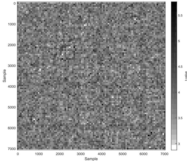
**Figure 5:** Second-order leakage for three-share version with four coefficients (masks enabled, 1 M measurements,  $t_{th} = 6.36$ ). Points with  $t$ -values above the threshold are highlighted red (none present).
