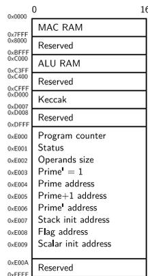
Figure 15: Memory arrangement of the SIKE processor.
