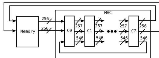
**Figure 9:** Pipeline with feedback to achieve  $\mathbb{F}_p$  operations.
