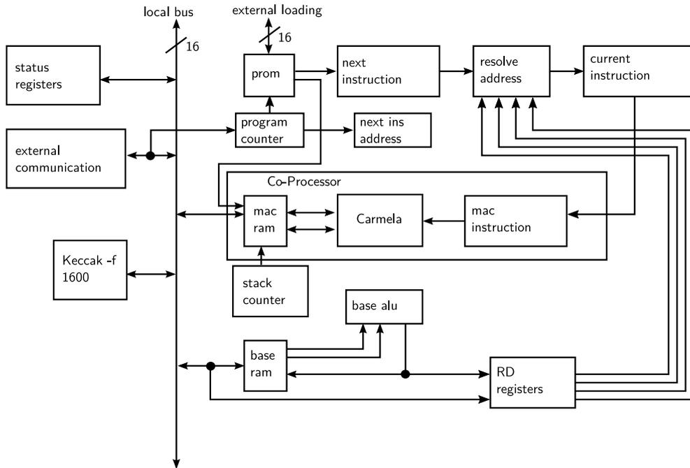
**Figure 3:** The high-level architecture of the SIKE processor.
