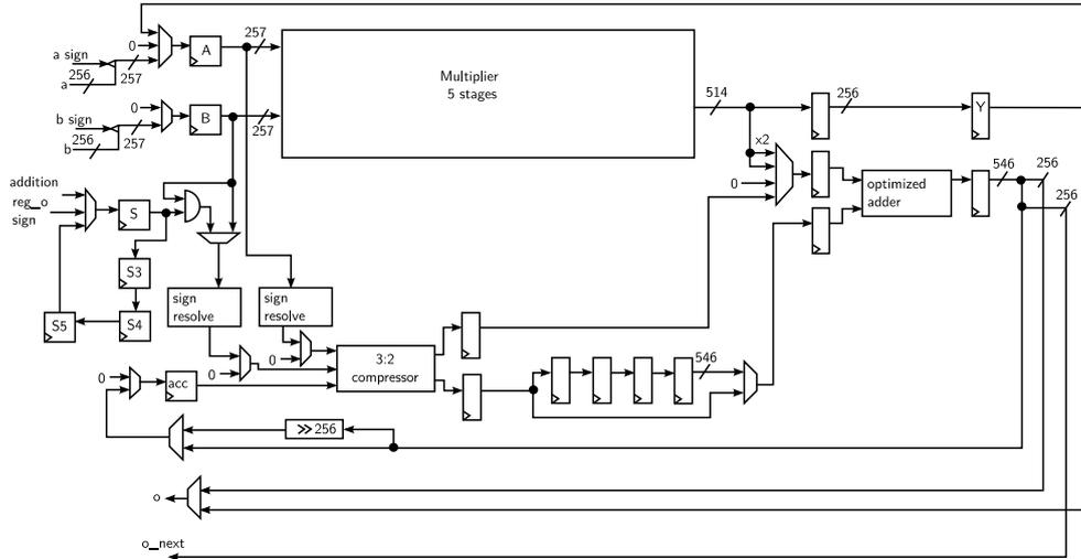
**Figure 8:** The 8-stage pipeline multiplier accumulator Carmela256.
