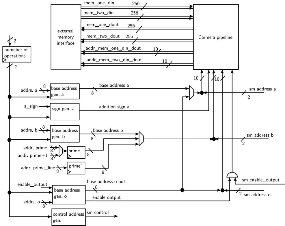
**Figure 10:** Carmela256 with address resolution and memory interfaces.
