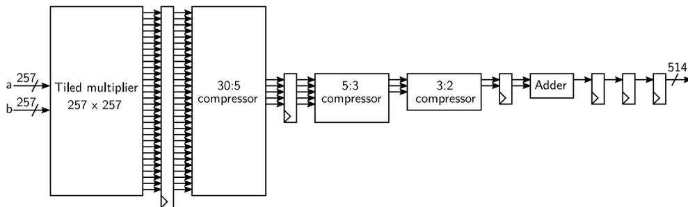
**Figure 6:** The 257-bit signed multiplier with compressor.
