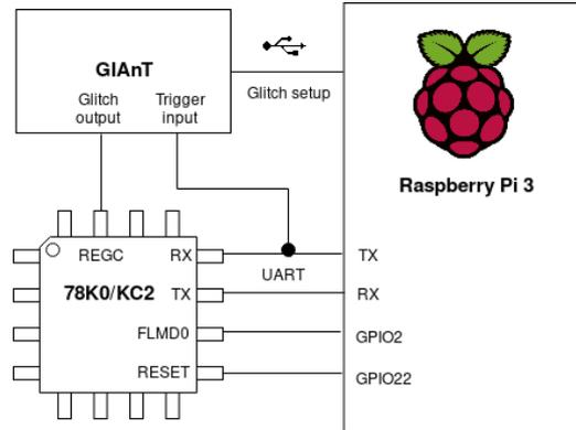
**Figure 3:** Our setup for the voltage glitching attack
