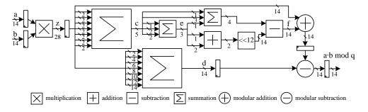
Figure 6: The architecture of modular multiplication.
