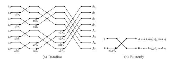
Figure 1: Dataflow of 8-point Low-Complexity NTT
