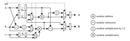
Figure 5: The architecture of butterfly unit.
