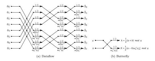
Figure 2: Dataflow of 8-point Low-Complexity INTT
