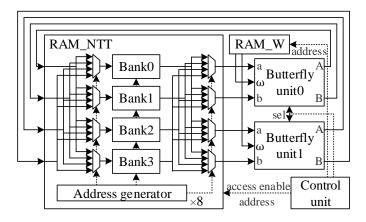
Figure 4: The architecture of NTT/INTT.
