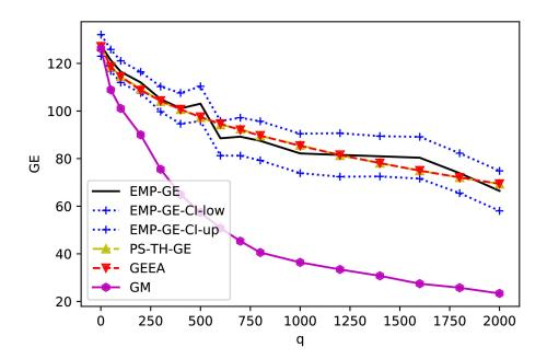
**Figure 1:** Comparison of four one-byte GE estimations (namely EMP-GE, PS-TH-GE, GEEA, and GM) of the template attack on SGII-1M data set. We also plot the 95% confidence intervals for EMP-GE, whose upper bound and lower bound are labeled respectively by EMP-GE-CI-up and EMP-GE-CI-low.
