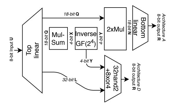
The Bottom matrix only depends on the multiplication of the 4-bit signal **Y** with some linear combination of the input signal **U**
