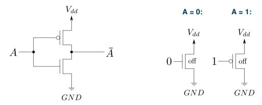
\*Active (conducting) transistors are replaced by ideal wires in this simplification.
