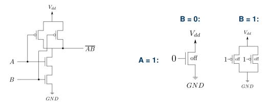
\*Active (conducting) transistors are replaced by ideal wires in this simplification.
