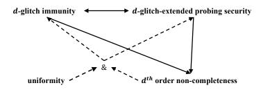
**Figure 2:** Illustration of the relations between different security notions for hardware security. The arrows indicate an implication relation. When the line is dotted, it is only valid for security order d = 1. The full lines are for any order d.
