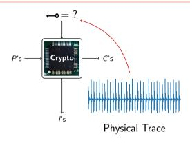
Leakage detection searches for dependency between manipulated data and physical traces.
