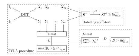
Figure 1: Leakage detection framework.
