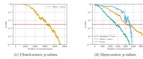
Figure 11: Leakage detection results: masked software AES implementation.
