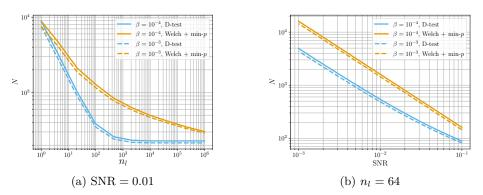
Figure 5: Number of traces N required to detect for a fixed false negative rate  $\beta$  on simulated traces with a density of  $\phi = 1$ , and varying trace length  $n_l$  and SNR.
