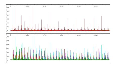
Figure 10: Monobit SNRs (on 50,000 traces) for the first operand of the MMM. Top: 32 SNR traces for each bit of *the least significant* 32-bit word. Bottom: 34 SNR traces for *all* the 12th bit of each 32-bit sub-word of the operand.
