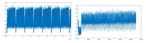
(a) Illustration of a part of the signal, with the succession of squaring and multiplication by MMM processing.
