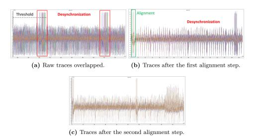
Figure 5: Alignment steps of the MMM pre-processing traces.
