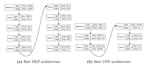
Figure 13: Best neural networks architectures on aligned traces.
