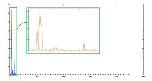
Figure 7: Icc Campaign – NICV scores w.r.t. time samples; in blue,  $\operatorname{seg}_{\operatorname{free}}$  values for  $\mathbf{L}^{\operatorname{sq.}}$ , in orange  $\operatorname{seg}_{\operatorname{free}}$  values for  $\mathbf{L}^{\operatorname{mult.}}$ , in magenta the exponent bit values for  $\mathbf{L}^{\operatorname{mult.}}$ .
