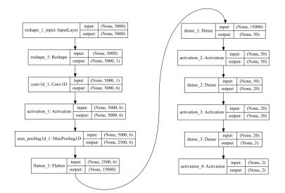
Figure 15: CNN architecture.
