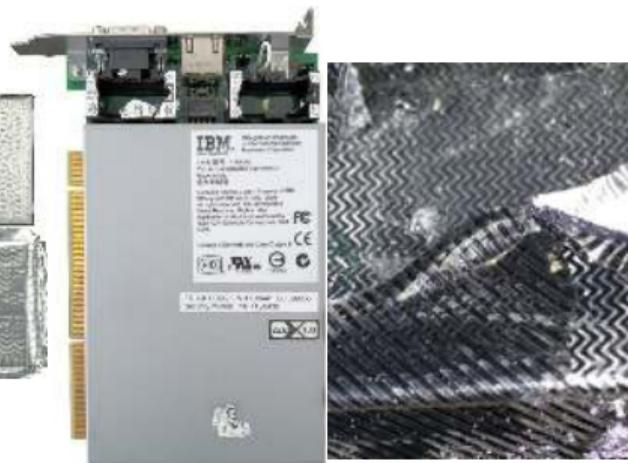
countermeasures: active meshes, obfuscation, light sensors, switches, potting, ...
