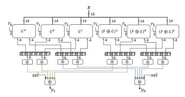
Figure 5: Illustration of the masked realization of the functions  $F^*/G^*$ .
