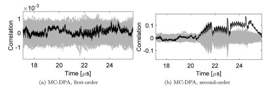
Figure 8: PRNG and initial masking enabled, Moments-Correlating DPA result targeting S-box no. 8 with model S-box no. 4, (a) first-order with  $10\,000\,000$  traces, (b) second-order with  $10\,000$  traces.
