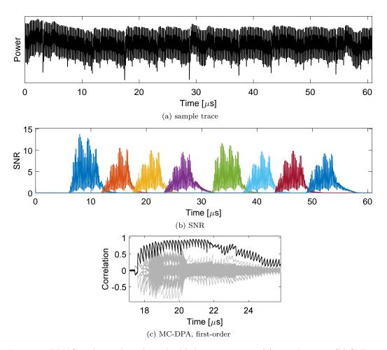
Figure 7: PRNG and initial masking disabled, 10 000 traces, (a) sample trace, (b) SNR curves based on 8 plaintext bytes with the order from left to right: byte no. 0, 4, 8, 12, 1, 5, 9, 13, (c) first-order Moments-Correlating DPA result targeting S-box no. 8 with model S-box no. 4, the black curve belonging to the correct key difference.
