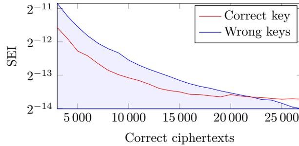
Figure 5: Attacks on 32-bit bitsliced SW AES, STM32 F3, detection countermeasure. SEI of the correct key ( $SEI_R$ ) vs. best SEI for a wrong key ( $SEI_W^*$ ) for  $N$  correct encryptions. 22 000 correct ciphertexts were required, stemming from about **130 000** faulted encryptions.
