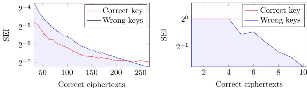
(a) ATXmega 256A3: 220 correct ciphertexts stemming from about 1 000 faulted encryptions are required. (b) ATXmega 128D4: 5 correct ciphertexts stemming from about 1 300 faulted encryptions are required.
