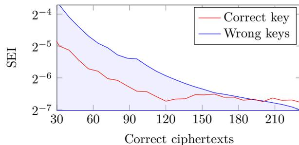
(c) ATXmega 128D4,  $t=66$ . 180 correct ciphertexts were required, stemming from about **46 000** faulted encryptions.
