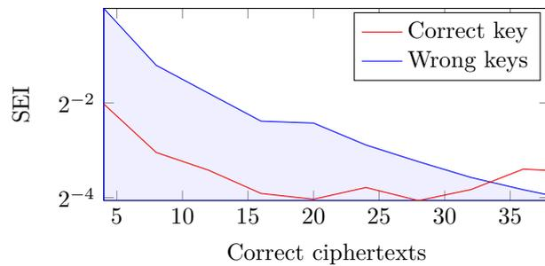
(b) ATXmega 128D4,  $t=22$ . 34 correct ciphertexts were required, stemming from about **9 000** faulted encryptions.
