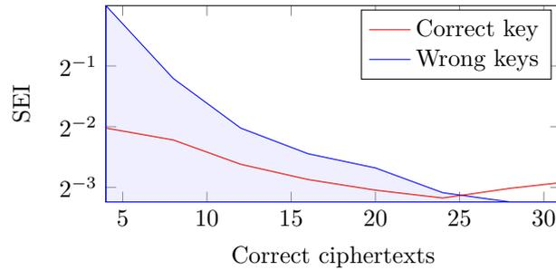
(a) ATXmega 128D4,  $t=11$ . 25 correct ciphertexts were required, stemming from about **6 500** faulted encryptions.
