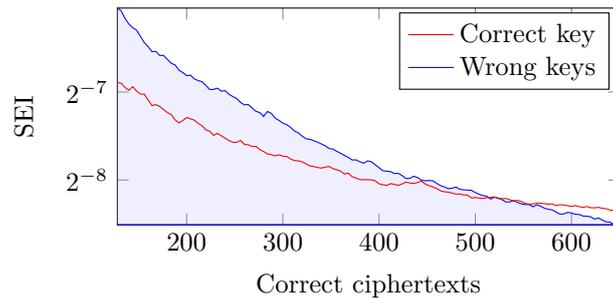
Figure 6: Attacks on HW AES co-processor, ATXmega 256A3, detection countermeasure. SEI of the correct key ( $SEI_R$ ) vs. best SEI of a wrong key ( $SEI_W^*$ ) for  $N$  correct encryptions. 550 correct ciphertexts were required, stemming from about **800** faulted encryptions.
