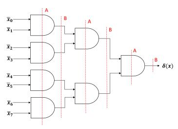
**Figure 15:** Circuit for the shared Kronecker delta function  $\delta(x)$  for n=8
