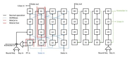
Figure 6: State and Key Array
