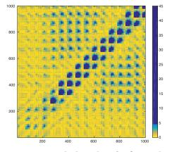
**Figure 11:** Non-specific bivariate leakage detection test on 15 clock cycles of a first-order protected AES. Left: 1 million traces. Right: 45 million traces.
