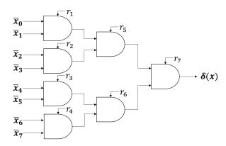
**Figure 4:** Circuit for the shared Kronecker delta function  $\delta(x)$  for n=8
