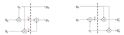
**Figure 16:** First-order Boolean to multiplicative (left) and multiplicative to Boolean (right) conversion circuits with intermediate probes
