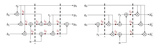
**Figure 17:** Second-order Boolean to multiplicative (left) and multiplicative to Boolean (right) conversion circuits with intermediate probes
