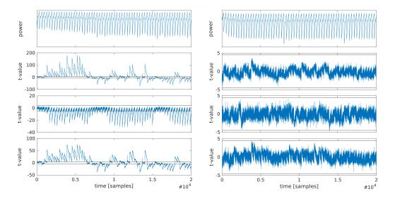
**Figure 9:** Non-specific leakage detection test on 2.5 rounds of encryption of a second-order protected AES. Left: PRNG off; 12 000 traces. Right: PRNG on; 50 million traces. Rows(top to bottom): exemplary power trace, first-order, second-order, third-order t-value.
