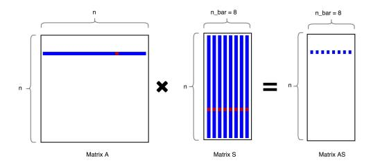
Figure 5: Concept of the multiplication of one row of  $\bf A$  with  $\bf S$  effectively. Blue entries are affected by one function call, red entries are loaded during one iteration.
