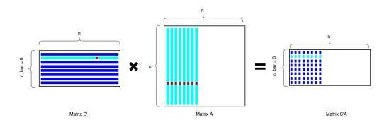
Figure 6: Concept of the multiplication of 8 columns of  $\bf A$  with  $\bf S'$  effectively. Blue and light blue entries are affected by one function call, light blue entries are loaded by one entire loop, red entries are loaded during one iteration.
