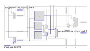
(a) An RO as implemented during compilation in the LUTs of an ALM of the Intel Cyclone V SoC
