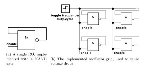
Figure 4: Schematics of the RO implementations
