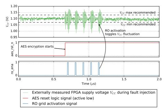
Figure 9: Trace of FPGA supply voltage *VCCINT*, measured externally with an oscilloscope during a single fault injection attempt
