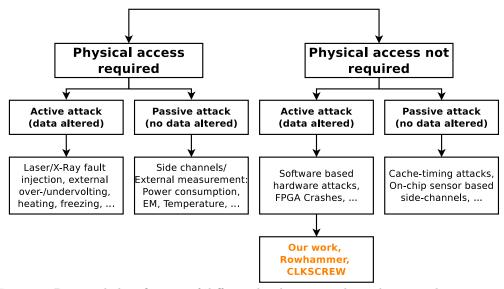
Figure 2: Proposed classification of different hardware attacks with our work categorized as an active attack, that does not require physical access to the attacked device
