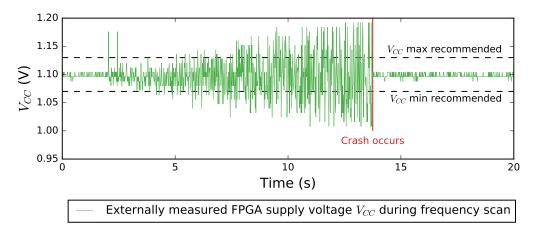
Figure 5: Trace of FPGA supply voltage *VCCINT*, measured externally with an oscilloscope during a frequency sweep leading to a crash of the device
