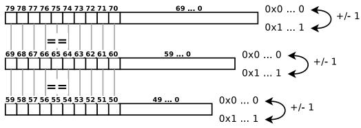
Figure 7: Simple adder design to evaluate fault attack vulnerability
