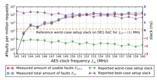
Figure 13: Total measured fault injection rates  $F_{\text{tot}}$  and measured injection rate of faults usable in DFA  $F_{\text{DFA}}$  as well as setup slacks reported by Quartus STA for different AES operating clock frequencies  $f_{\text{op}}$  with preserved design placement but remaining routing randomization on the DE0-Nano-SoC
