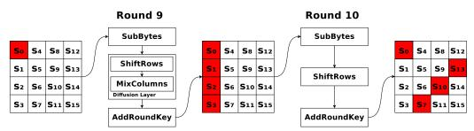
Figure 3: Propagation of a faulty byte in the input of the 9th round of the AES algorithm
