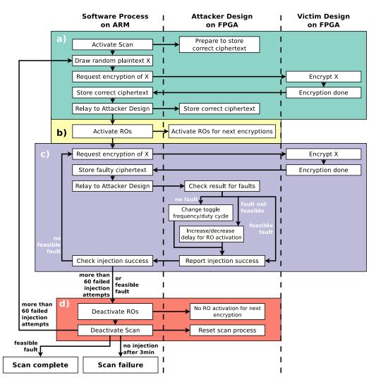
Figure 8: Flowchart of the calibration algorithm to find the appropriate parameters for injecting faults at the desired moment
