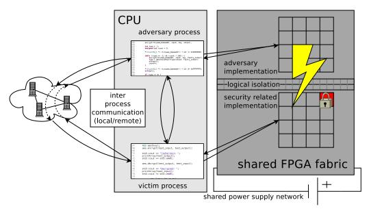
Figure 1: Overview of the threat model considered in this work: Attacker and victim share an FPGA resource with a common power supply network, but isolated, logically disconnected partitions on the fabric
