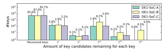
Figure 12: Amount of key candidates remaining for each DFA key recovery attempt on 5000 randomly drawn AES keys on three different DE1-SoC boards
