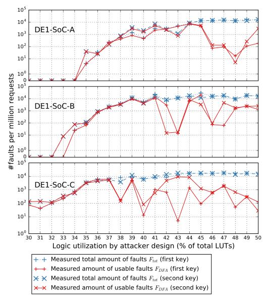
Figure 11: Total measured fault injection rates  $F_{\text{tot}}$  and measured injection rate of faults usable in DFA  $F_{\text{DFA}}$  with respect to the amount of logic utilization (percentage of total LUTs) by the attacker design for three different Terasic DE1-SoC boards and two different random encryption keys
