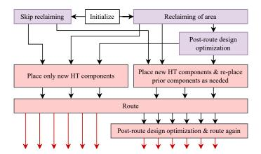
**Figure 9:** Extended attack techniques. The orchestration fans out into 12 different, fully automated modes for advanced HT insertion, as indicated by dark-red arrows. Pre-attack steps are highlighted in purple and attack steps for physical integration in light-red.
