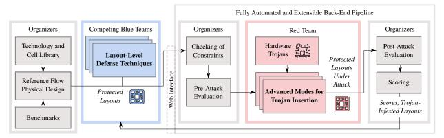
**Figure 2:** Overview of the end-to-end framework for benchmarking of layout-level defenses versus advanced HT insertion.
