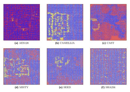
**Figure 13:** Layout illustrations for all benchmarks. Shown are regular cell instances in blue, cell assets in dark-yellow, exploitable regions in red, and remaining open sites in grey, respectively. Different dimensions result in varying levels of detail visible in these fixed-size plots.
