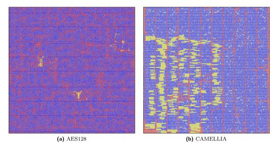
**Figure 4:** Layout illustrations for selected benchmarks. Shown are regular cell instances in blue, cell assets in dark-yellow, exploitable regions in red, and remaining open placement sites in grey, respectively. Different dimensions result in varying levels of detail visible in these fixed-size plots. All benchmarks are also illustrated in Fig. 13 (App. F).
