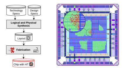
**Figure 1:** The threat of fabrication-time HT insertion. (Left) Simplified IC design flow and supply chain with the adversary and the attack highlighted. (Right) An exemplary HT attack on an AES core in an actual IC [PP22]. HT logic is shown in red, selected regular cells in green, routing in blue/brown, and peripherals in purple.
