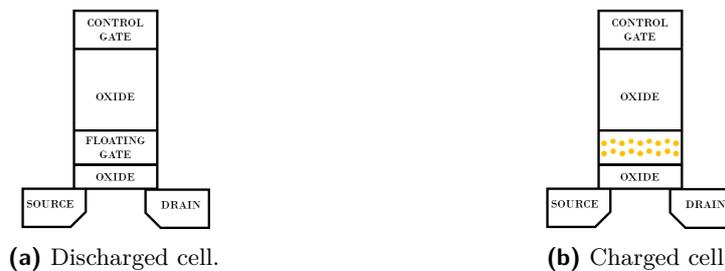
**Figure 1:** Cross-sectional view of a floating gate transistor.
