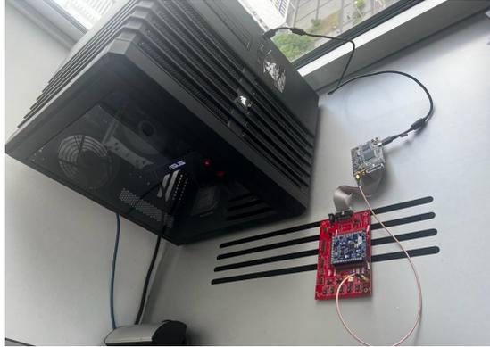
**Figure 6:** Experimental workbench used for our fault injection attack; it contains an STM32F4 target board mounted on the UFO board (red), a ChipWhisperer CW308, two SMA cables, and a USB cable.
