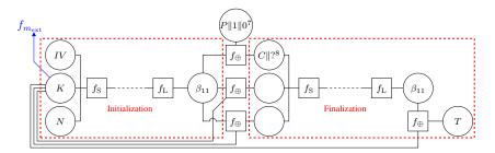
**Figure 7:** The factor graph at state level covering a full ASCON-128 encryption, with empty associated data and seven-byte plaintext (observation factors omitted).
