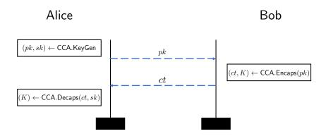
Figure 2: Key-Exchange protocol using IND-CCA secure Kyber KEM
