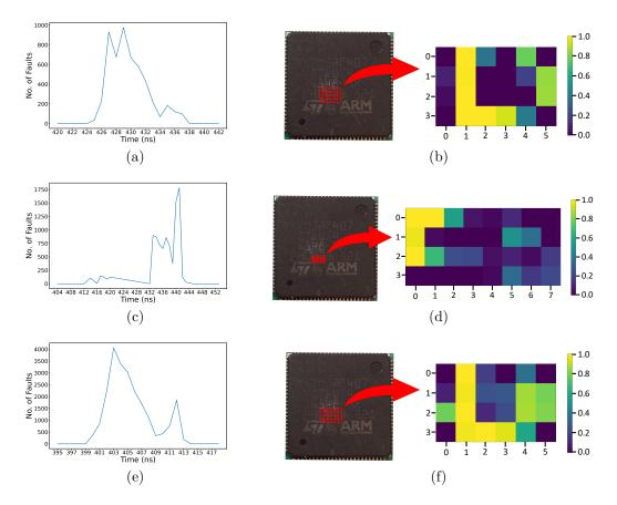
**Figure 8:** EMFI Results for Sign\_Fault\_NTT\_C on deterministic signing procedure (a,b) and Sign\_Fault\_NTT\_Y on probabilistic signing procedure (c,d) and Verification-Bypass (e,f) for Dilithium3. (a,c,e) denotes Sensitive Time window, while (b,d,f) denotes best fault repetability achievable at different sensitive locations (XY) for the corresponding attacks.
