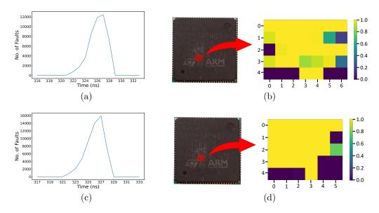
**Figure 7:** EMFI Results for Kyber-Key-Recovery (a,b) and Kyber-Message-Recovery (c,d) for Kyber768. (a,c) denotes sensitive time window, while (b,d) denotes best fault repetability achievable at different sensitive locations (XY) for the corresponding attacks.
