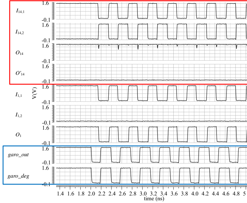
Figure 13: The simulated waveforms with feedback polynomial f(x) = x^{15} + x^{14} + x + 1 .
