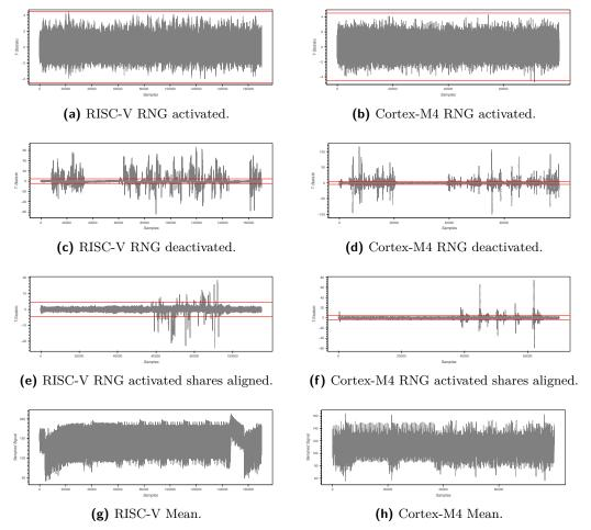
**Figure 7:** First-order t-test results of a Keccak-f[800] round. The  $\pm 4.5$  threshold is marked by red lines. Experiments with RNG active use 1M traces, with RNG inactive use 10k traces, and with aligned share evaluations use 100k traces.
