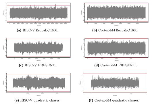
**Figure 8:** First-order *non-specific*, *fixed vs. random* t-test results on RISC-V and Cortex-M4 cores with 1M traces. The  $\pm 4.5$  threshold is marked by red lines.
