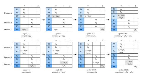
**Figure 5:** Outputs  $c_0$  and  $c_1$  of the Toffoli gate. In this masking, registers R0-R2 belong to domain A, R3-R5 belong to domain B, and R6 is a temporary register in domain T.
