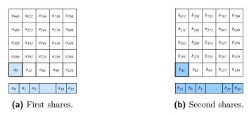
**Figure 6:** Placement of the first (left) and second (right) shares represented as matrices of  $5 \times 5$  lanes. The first 32-bit lane of each share is detailed in the lower part of the figure with their respective (shifted) bit indices. The first share is denoted by a and the second by b where we use subscript to indicate the separate bits.
