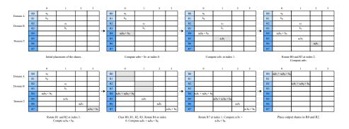
**Figure 4:** Methodology for d + 1 shares. In this masking, registers R0-R1, R2-R3 belong to domain A and B respectively and R4-R7 are temporary registers in domain T.
