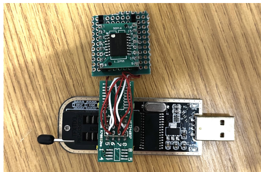
Figure 3: Dumping BMC firmware with a flash programmer.
